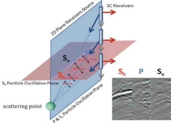
Figure 2: The elastic, scattered wave field seen by the 3C receivers.
