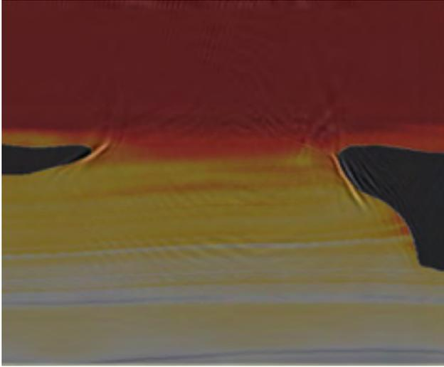
Figure 8: A vertical section through the 3D image cube from the North-West to the South-East, intersection the two main salt bodies, overlain by the true velocity model. The salt bodies are the two dark-grey objects to the left and to the right. Only sediment velocities are used for this image, and taking care to eliminate the shots propagating through the salt.
