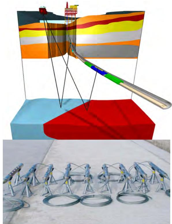
**Figure 1: On the top, an illustration of the geometry used for VSP data acquisition. The well is instrumented with acoustic sensors (on the bottom).**
