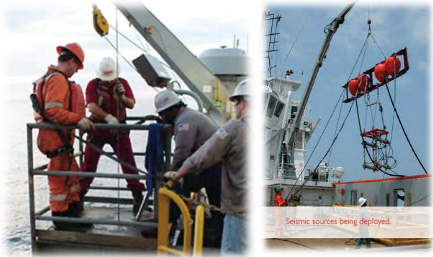
**Figure 2: Deploying receivers (left) and an acoustic source (right) at an offshore location.**
